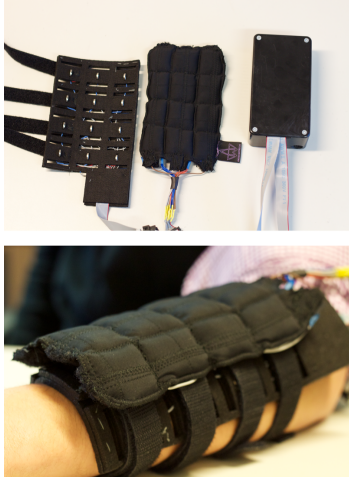
Figure 1: The TaSST. The top image shows the output layer, the input layer, and the control box.
