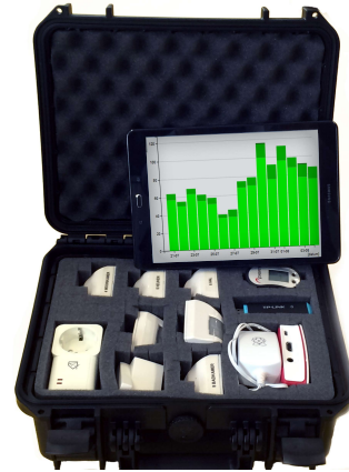
Figure 1: The Hipperbox consisting of a Raspberry Pi, a set of sensors and a tablet.
